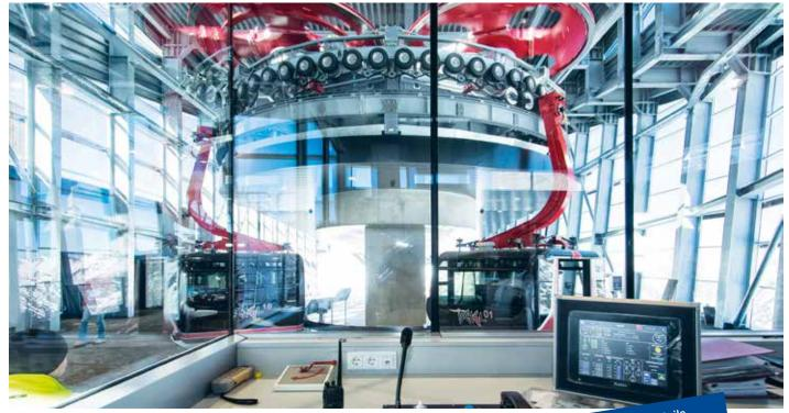
World first: The cabins on the Pardatschgrat 3S can draw power from a carriage dynamo – to heat the seats, for example.
