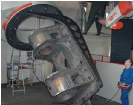
The IGM welding robot can handle parts of up to 5 tonnes in weight
