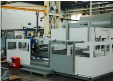
DMC 200 U universal milling center with shuttle table
