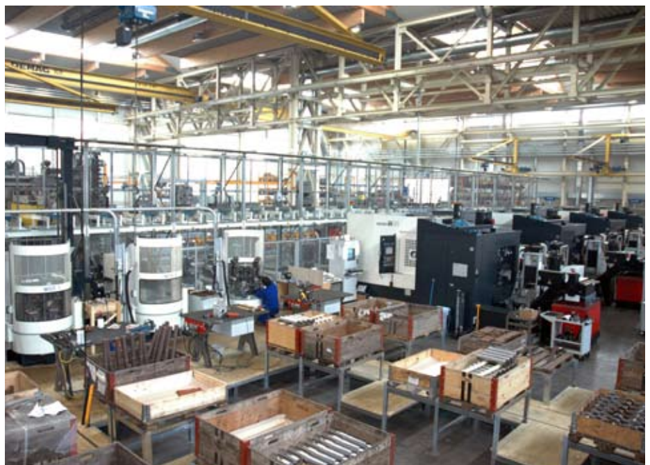
The four interlinked Makino A81 machining centers (to the right of the photo) with three loading and unloading stations (in white) and component set-up area (front)
