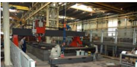
IGM-IBS drilling robot for weld seam preparation
