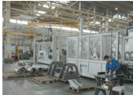
SHW Power Speed 5 traveling column milling center with 16 m travel.
