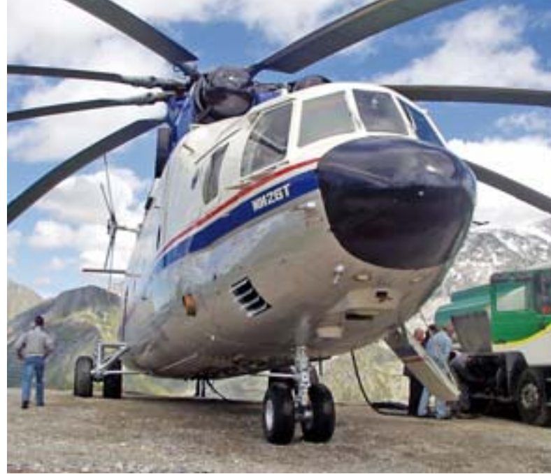
An Mi26-T, the world's heaviest freight helicopter manufactured in series, was used for the installation work. It has eight rotor blades, two 8350kW engines (in total 22,400 PS) and measures 46 m in length. With a take-off weight of 56 tonnes, it can transport up to 20 tonnes of freight.
