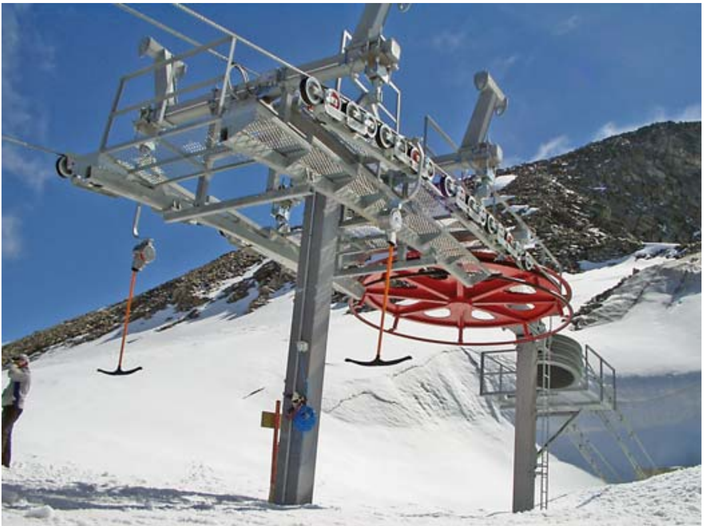
Bottom terminal of Kaserer 1 below the Hintertux Glacier at an altitude of 2705 m: at the front the mast for guy rope tensioning, behind it the drive with 230 kW DC motor and hydraulically operated platform for relocating the grips.
