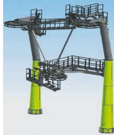
Unique technical feature: The twisted curve tower structure on the Krupová surface lift
