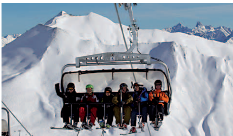
The Masnerkopf lift in Serfaus is the first to be equipped with the new FMV footrest system from Doppelmayr. The chairs feature seat dividers and a central footrest for each seat. The restraining bar is manually operated and locks when properly closed. The lock is automatically deactivated in the top station; only then is it possible to open the restraining bar, which again is performed manually. There is no monitoring of the chair locking operation.
