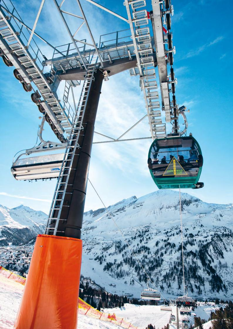
Thanks to its high flexibility, this ropeway system can be optimally adapted to different requirements. Within a given system, all carrier mixes are generally possible, depending on the season, the prevailing weather conditions and customer requirements. In summer, for example, there may be a need to run cabins only.
